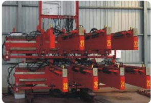
海洋钻机可调节套管指梁 Adjustable casing fingerboard for offshore drilling rig
