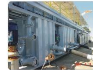
钻井泥浆净化系统 Drilling mud purification system
